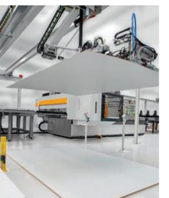
The Winstore automated magazine stacks sheets of different sizes and materials, including mixed ones, with no need for operator intervention. The reorganisation of sheet magazine and stacking can be carried out automatically, out of working hours.
